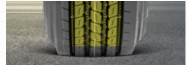
Evenly distributes grounding pressure, and irregular wear resistance
