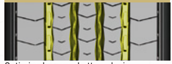
Optimized groove bottom design
